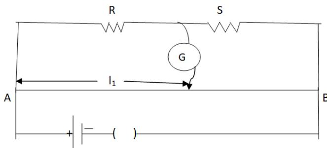
An unknown resistance  $X$  is now connected in parallel to the resistance  $S$  and the balance point is found at a distance  $l_2$ . Obtain the formula for  $X$  in terms of  $l_1$  and  $l_2$  and  $S$ .
