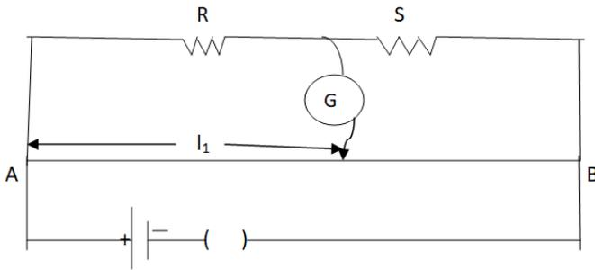
In a metre bridge with  $R$  and  $S$  in the gaps, the null point is found at 40 cm from A. If a resistance of  $30 \Omega$  is connected in parallel with  $S$ , the null point occurs at 50 cm from A. Determine the values of  $R$  and  $S$ .
